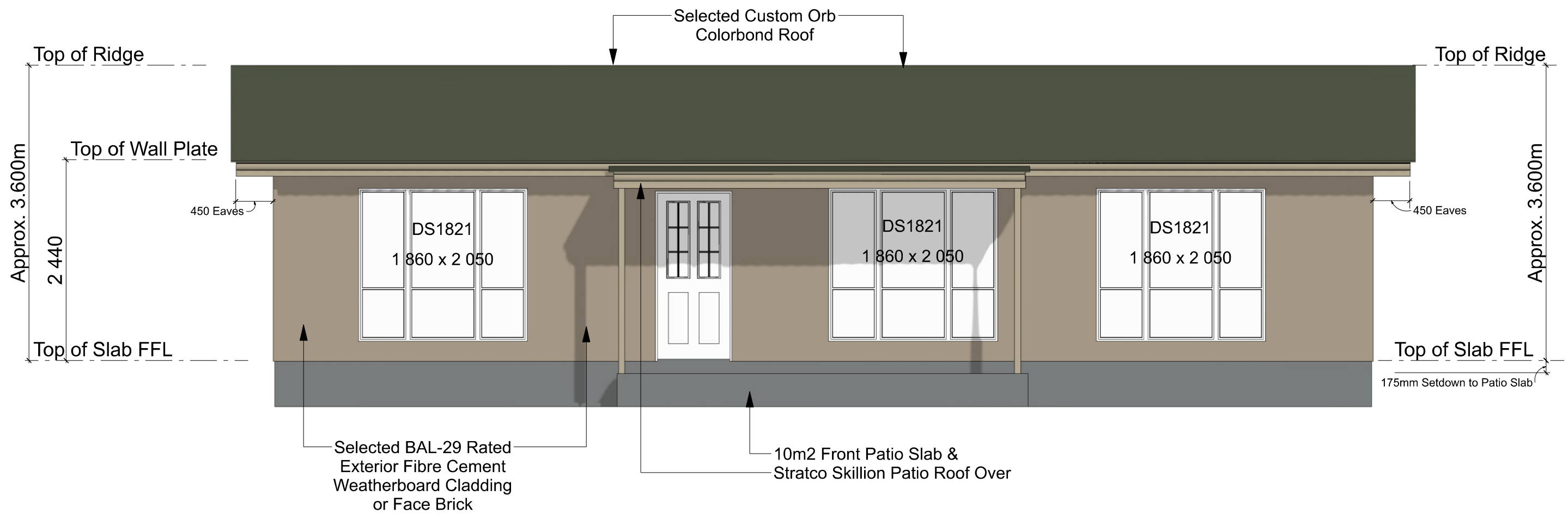
FRONT ELEVATION - 1 Bedroom - 93m 2 - Residence SCALE: 1:50
